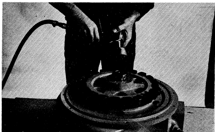
Fig. 31. Disassembly of Spider drive using Special Tool.
