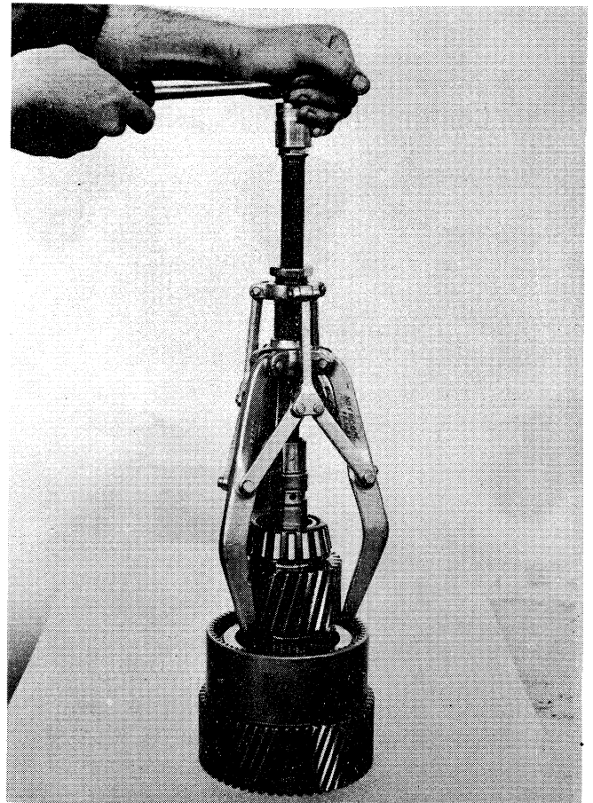
Fig. 20 . Pulling the Rear Bearing Cone from the Forward Clutch Shaft.
