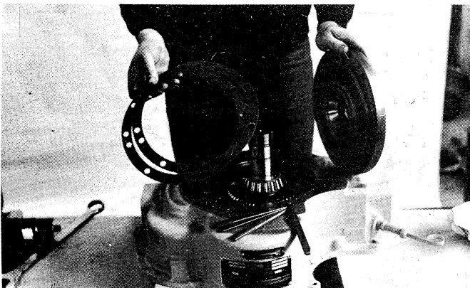
Fig. 36 Installing Shims and Input Bearing support.
