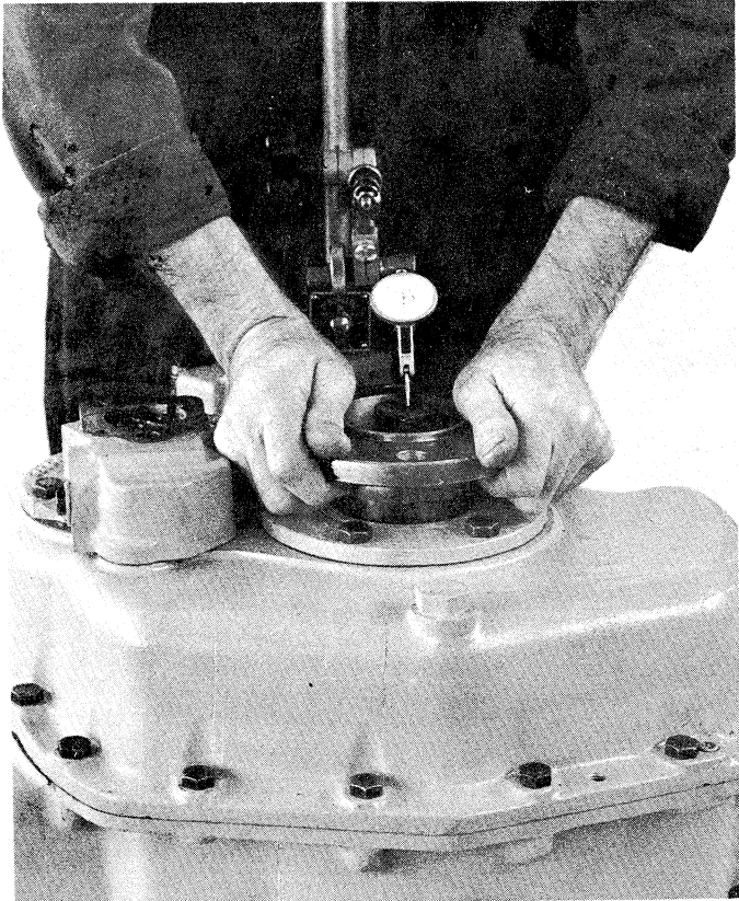
Fig. 43. Applying pulling force while checking end play of Input Shaft with dial indicator.
