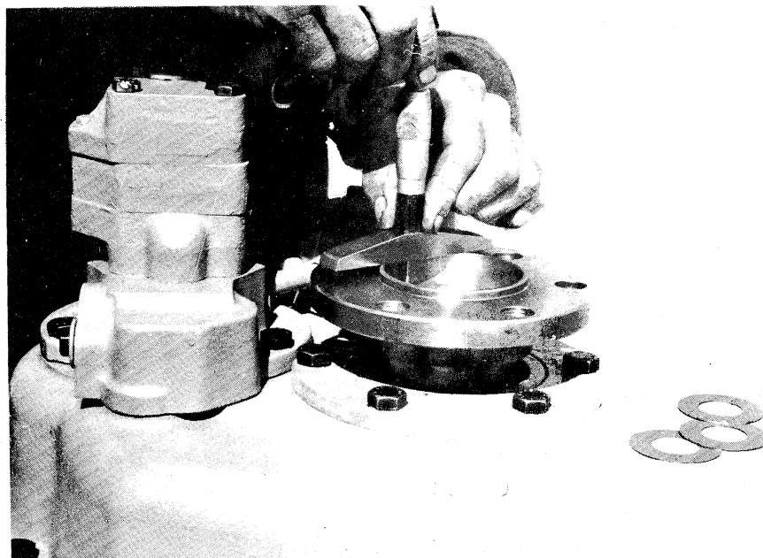
Fig. 48 Measuring Shim space between output shaft and retainer face of the flange.
