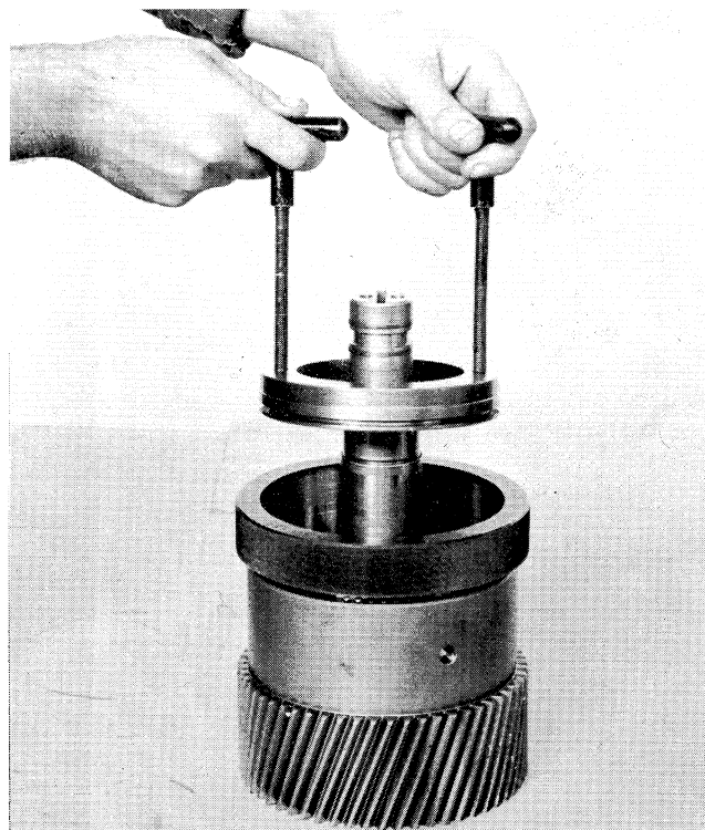
Fig. 30 . Removing clutch piston assembly using special tools.
