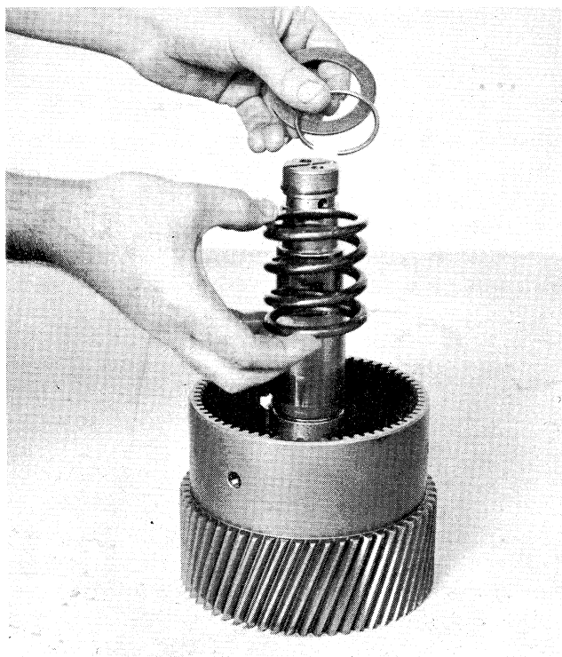
Fig. 27 . Removing clutch release spring and retaining parts.
