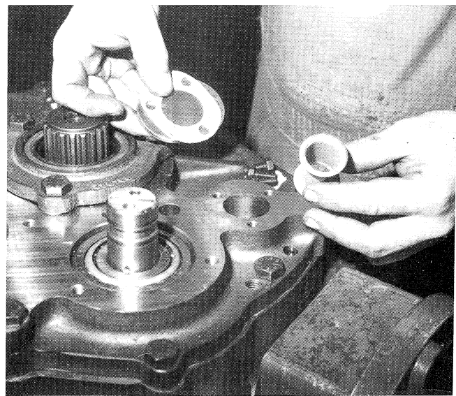
Figure 6-4. Pump Suction Filter Screen and Cover Plate Removal.
