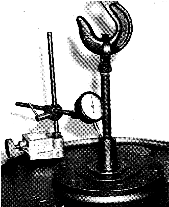
Figure 9-9. Applying Pulling Force While Dial Indicating End Play of Input Shaft.
