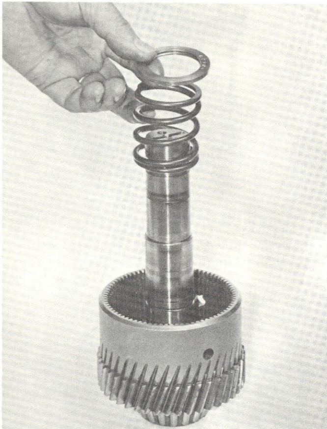
Figure 21. Removing Clutch Piston Return Spring and Retainer.
