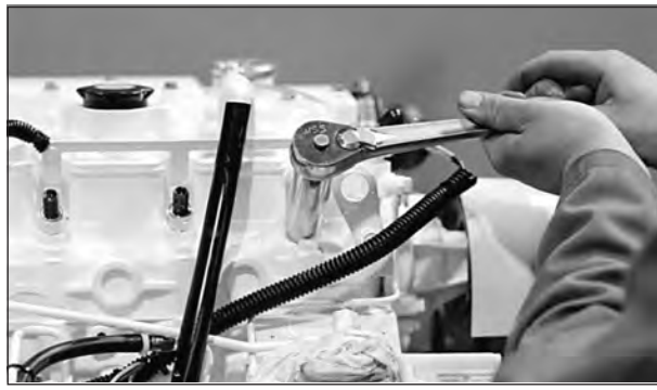
Figure 17: Reinstall injector. Torque to proper tightness.
