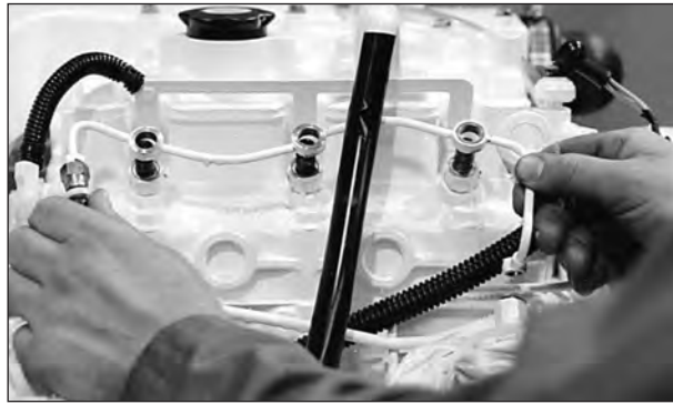
Figure 14: Remove return line.
