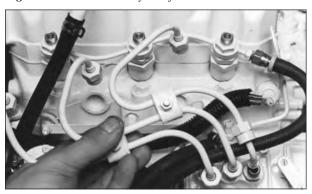
Figure 8: Remove delivery lines.
