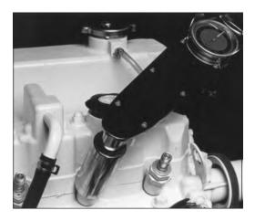
Figure 13: Reinstall injector. Torque to proper tightness.
