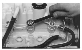
Figure 9: Remove return line nuts.
