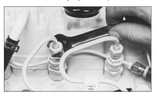
Figure 7: Remove delivery line flare nuts.
