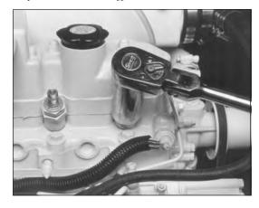
Figure 11: Unscrew injector.
