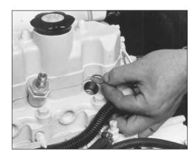
Figure 12: Remove and replace copper sealing washer.
