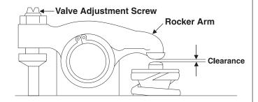
Figure 8: Valve Adjustment
