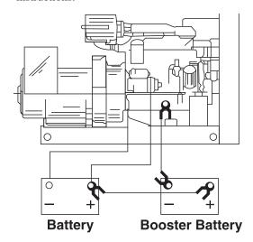
Figure 16: Booster Battery Connections
