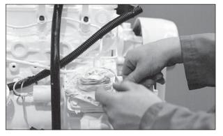
Figure 13: Cover lines, inlets and injection pump outlets.
