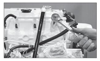
Figure 16: Unscrew injector.
