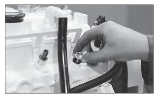
Figure 17: Remove and replace copper sealing washer.
