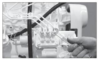
Figure 11: Remove delivery line flare nuts.
