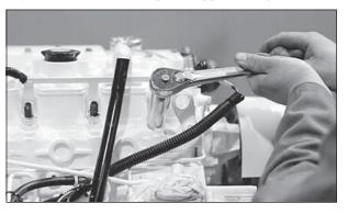
Figure 18: Reinstall injector. Torque to proper tightness.
