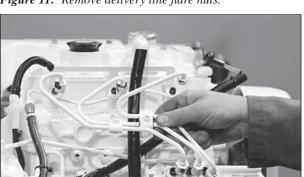
Figure 12: Remove delivery lines.
