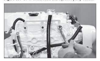
Figure 14: Remove return line nuts.
