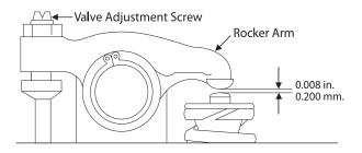
Figure 8: Valve Adjustment
