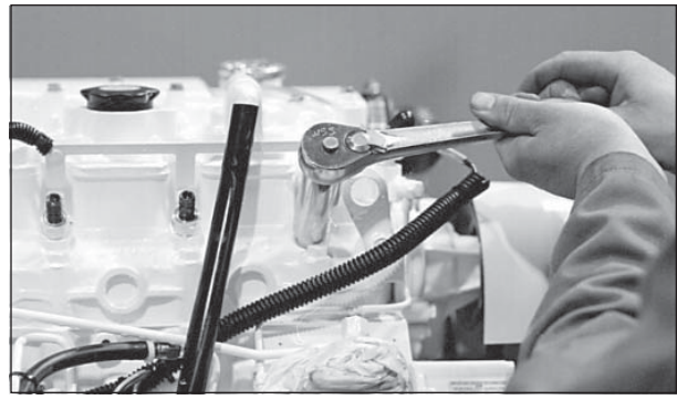
Figure 16: Reinstall injector. Torque to proper tightness.
