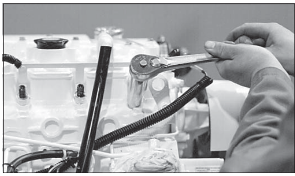
Figure 17: Reinstall injector. Torque to proper tightness.
