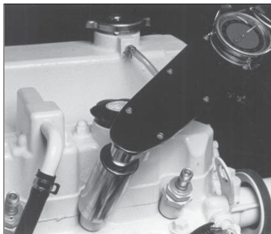
Figure 18: Reinstall injector. Torque to proper tightness.
