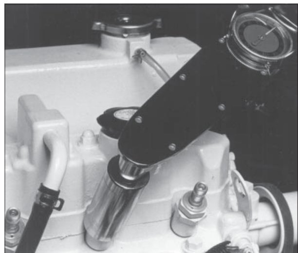
Figure 18: Reinstall injector. Torque to proper tightness.
