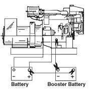
Figure 20: Battery connections.
