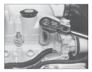
Figure 16: Unscrew injector.
