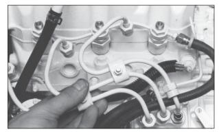
Figure 13: Remove delivery lines.
