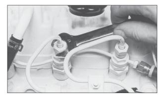
Figure 12: Remove delivery line flare nuts.
