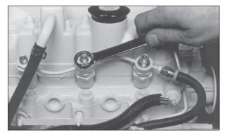
Figure 14: Remove return line nuts.
