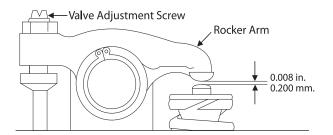
Figure 9: Valve Adjustment
