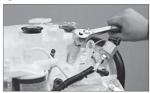
Figure 18: Unscrew injector.
