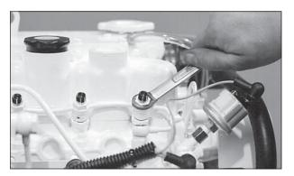
Figure 16: Remove return line nuts.
