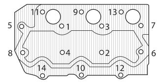
Figure 9: 673M Head Torque Sequence
