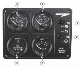
Figure 6-B: Series 3 Generator Control Panel
