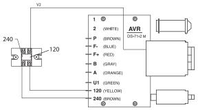
Figure 25: Control Terminal Board, 120 Volt Output
