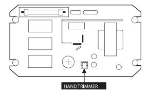
Figure 31: Hand Trimmer Location on AVR.
