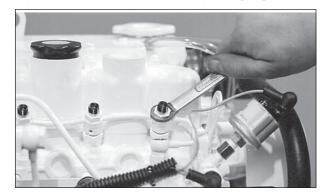
Figure 15: Remove return line nuts.
