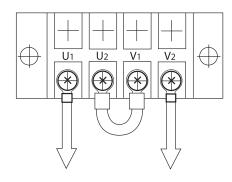
Figure 28: Output Terminal Board, 240 Volt Output
