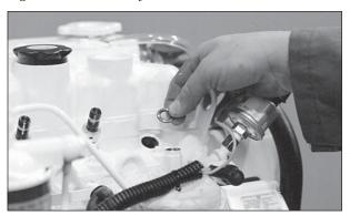
Figure 18: Remove and replace copper sealing washer.
