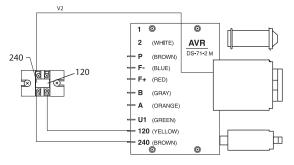
Figure 27: Control Terminal Board, 240 Volt Output b. Connect U2 to V1 on the output terminal board (Figure 28).
