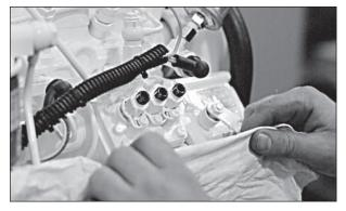
Figure 14: Cover lines, inlets and injection pump outlets.
