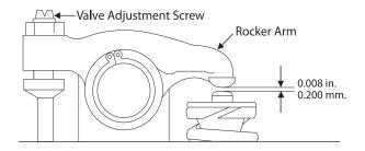
Figure 10: Valve Adjustment
