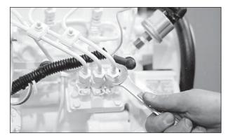
Figure 12: Remove delivery line flare nuts.
