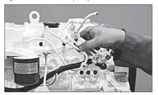
Figure 13: Remove delivery lines.
