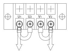
Figure 26: Output Terminal Board, 120 Volt Output
