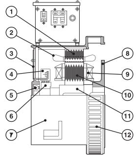
Figure 23: Generator Components.
