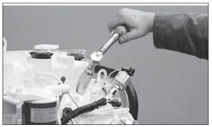
Figure 19: Reinstall injector. Torque to proper tightness.
