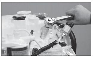
Figure 17: Unscrew injector.
