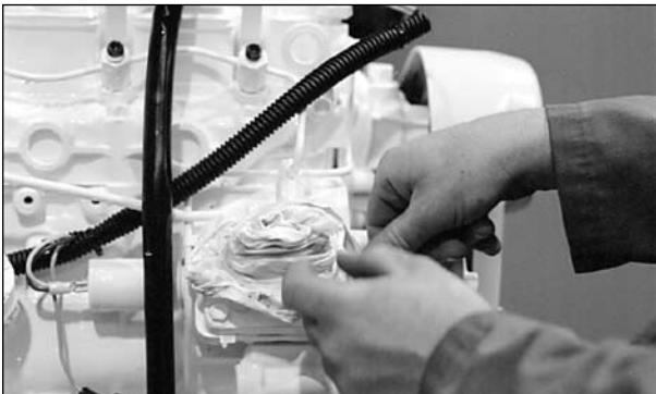
Figure 13: Cover lines, inlets and injection pump outlets.
