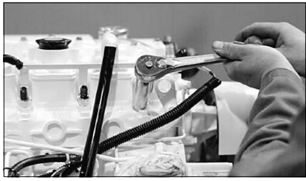
Figure 18: Reinstall injector. Torque to proper tightness.
