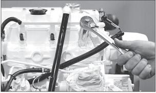
Figure 15: Unscrew injector.
