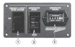
Figure 4-A: Series 1-B Generator Control Panel
