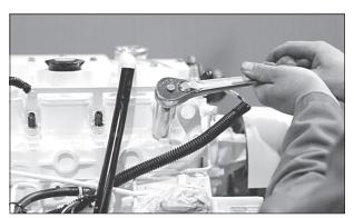
Figure 17: Reinstall injector. Torque to proper tightness.
