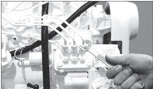
Figure 10: Remove delivery line flare nuts.
