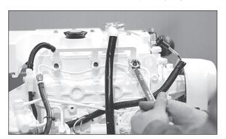
Figure 13: Remove return line nuts.
