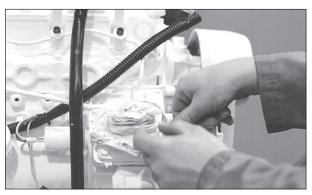
Figure 12: Cover lines, inlets and injection pump outlets.
