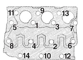
Figure 7: 843N Head Torque Sequence
