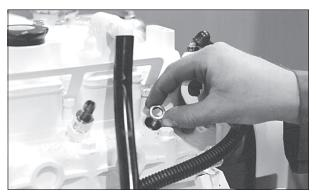
Figure 16: Remove and replace copper sealing washer.
