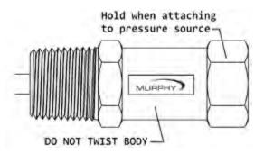
Transmitters require no special mounting hardware and can be mounted in any plane with negligible position error.
