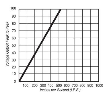
Note: Tested at 1000 I.P.S. 20 pitch gear 0.005 gap and 100K OHM load.
