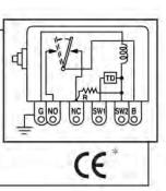
M4264 Series Detects loss of magneto/CD ignition output and transfers contacts for customer use. Contacts 10 amps; 48 VAC/VDC. M42641CD transfers SPDT dry contacts when tripped.
