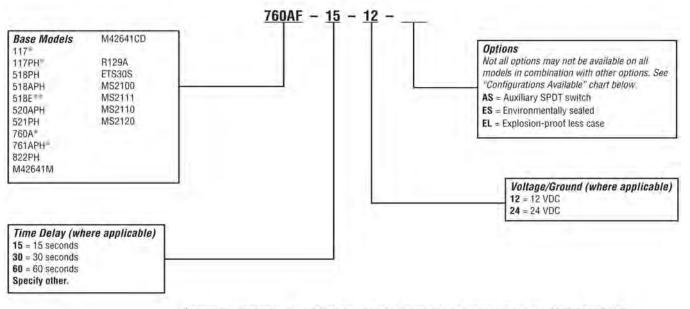
\*Add the letter "F" to the base model to indicate an inline fuse instead of a base mounted fuse. Example: 760AF, 761APHF, 117F \*\*12 Volt negative ground version only.
