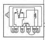
518APH Allows for SWICHGAGE<sup>®</sup> and/or N.C. contacts to be wired "Closed Loop" (in series). Any contact open or SWICHGAGE<sup>®</sup> contact close in the circuit shunt trips the 518APH. Specify 12 or 24 VDC. Contacts 10 amps 24V. 14 amp fuse.
