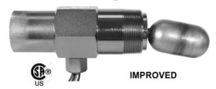
**LS200** Liquid Level Switches with 2" NPT mounting are float activated to operate an electrical SPDT snap switch (optional DPDT on some models) for alarm or shutdown of an engine or electric motor. The LS200 connects directly into the vessel wall and can be used with a Murphy weld collar (P/N 15050375) or Murphy external float chamber (P/N 15700799).
