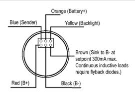
CAUTION: Devices containing solid state components can be damaged or caused to malfunction when used in systems which incorporate inductive loads (e.g. relays, solenoids, etc.) that can generate voltage spikes.
