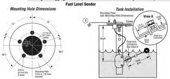
NOTE: When installing the fuel sender in a non-metallic tank using a single wire sender, another wire must be added from one of the sender mounting bolts to the battery ground (negative post). See 1 in the 'Tank Installation' illustration above.
