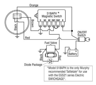
NOTE: Do not connect 117PH or power on TL7 to brown wire. Only use 518(A)PH or 760 Tattletale indicators. Pilot a relay with a flyback diode across the coil for loads pulling more current than rated.
