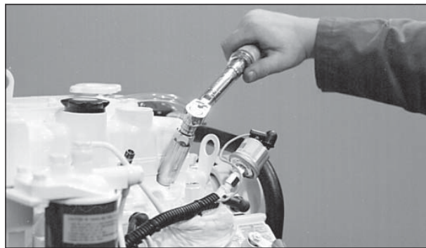
Figure 20: Reinstall injector. Torque to proper tightness.
