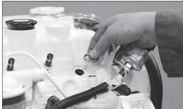
Figure 19: Remove and replace copper sealing washer.
